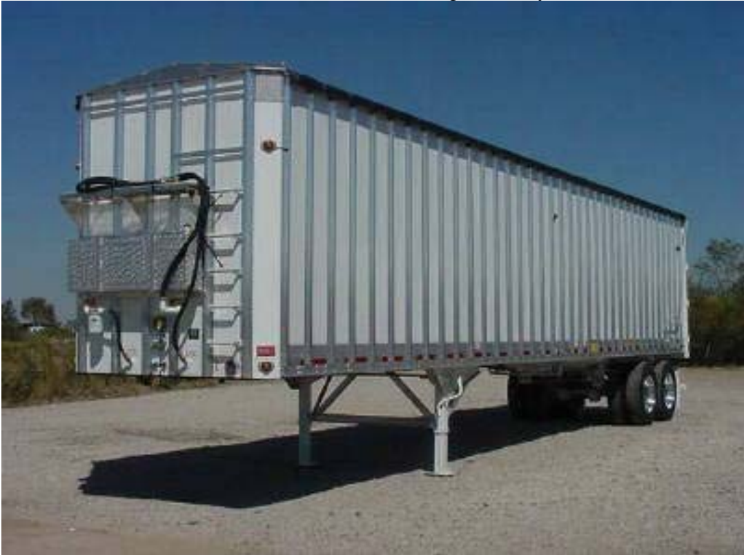
Live bottom semi-trailer – Often used for ground hay (Photo # 4)
