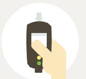
**ABORT TAMPER** - This message means that something is blocking the flow of air through the device. Blockage can be caused by items that have been blown into the device or by your hand covering the vent on the back of the device. Check for obstacles, remove them, and blow again.
